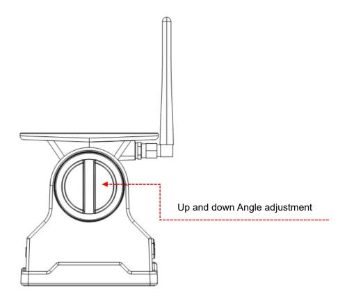
Loosen clockwise, adjust the corresponding angle, and fix counterclockwise.
