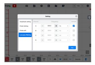
Figure 9-49 Low-pass Filtering Screen
