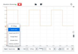
Figure 9-91 Signal Mode Setting Screen
