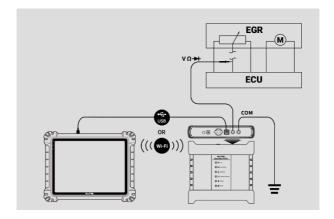
Figure 9-92 DC Voltage Connection Diagram
