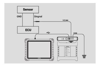
Figure 9-96 Triangle Waveform Connection Diagram
