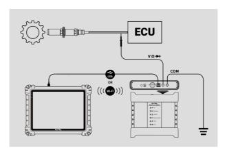
Figure 9-94 Square Wave Connection Diagram
