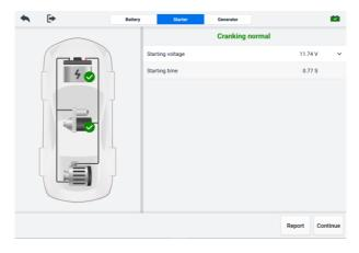
Figure 11-8 Starter Test Result Screen
