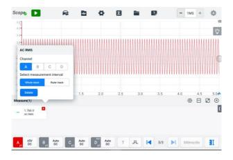
Figure 9-59 Measurement Setting Screen
