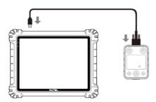
Figure 15-1 Connecting MaxiSys Tablet and Hand-held Inclinometer
