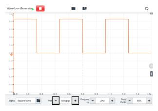
Figure 9-98 Voltage Setting Screen 1
