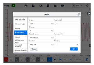
Figure 9-54 Pulse Width Settings Screen
