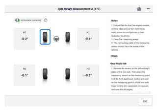
Figure 15-3 Ride Height Measurement Result Screen
