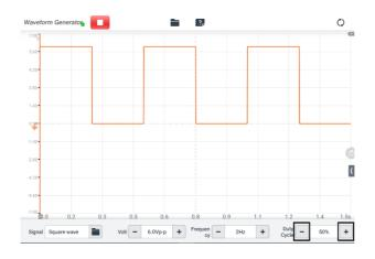
Figure 9-104 Duty Cycle Setting Screen 1
