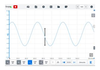
Figure 9-36 Dragging Waveform or Moving Screen
