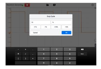
Figure 9-106 Duty Cycle Setting Screen 3
