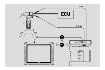
Figure 9-95 Square Wave (X+Y) Connection Diagram
