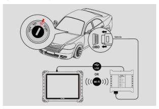
Figure 9-107 Connection Diagram
