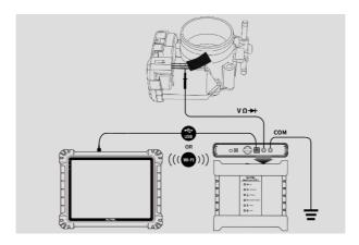
Figure 9-61 Connection Diagram
