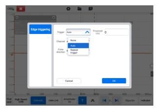
Figure 9-127 Trigger Mode Screen
