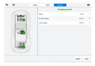
Figure 11-9 Generator Test Results Screen
