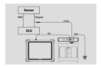
Figure 9-97 Arbitrary Waveform Connection Diagram
