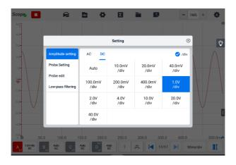
Figure 9-42 Amplitude Setting Screen (DC 1.0 V/div)
