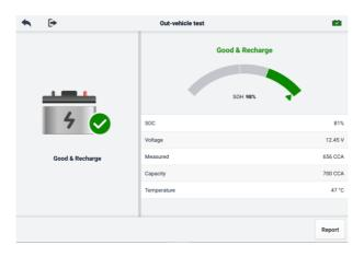
Figure 11-11 Out-vehicle Test Results Screen
