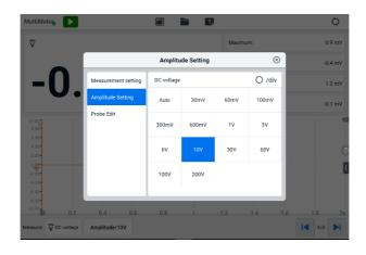
Figure 9-76 Amplitude Setting Screen (DC 10 V)
