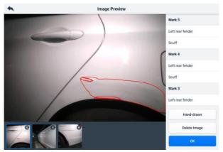
Figure 5-2 Vehicle Appearance Inspection Screen 1
