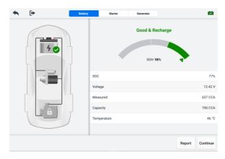
Figure 11-7 Battery Test Results Screen
