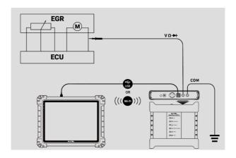
Figure 9-93 Actuator Drive Connection Diagram
