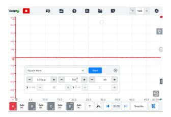
Figure 9-23 Waveform Generator Display Screen
