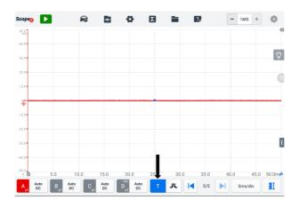
Figure 9-50 Trigger Point Screen
