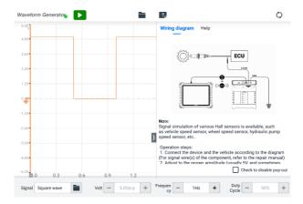
Figure 9-89 Wiring Diagram and Help Screen
