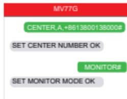
2. Switch the device to monitor mode by this command:**MONITOR#**
